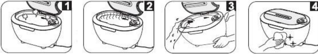
1. Do not turn on the washer without water inside. Turning on the washer without water can damage the washer.
